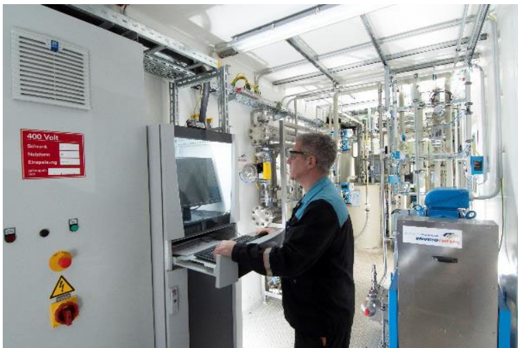
Image: In the ReSalt joint project, the fully automatic high-pressure osmosis system from EnviroChemie removes table salt from industrial water and concentrates it. ©image Covestro
