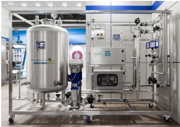
Image: PW storage and distribution system with ozonisation for a logistics centre and the hospital pharmacy of a group of hospitals in Ludwigsburg/Bietigheim.
