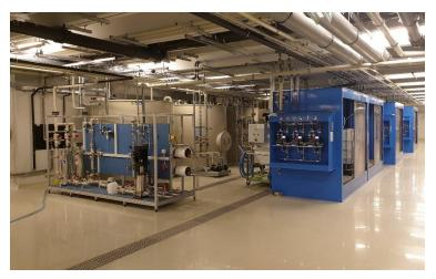
Image: Plant for chemical and physical wastewater treatment for a solar cell manufacturer.
