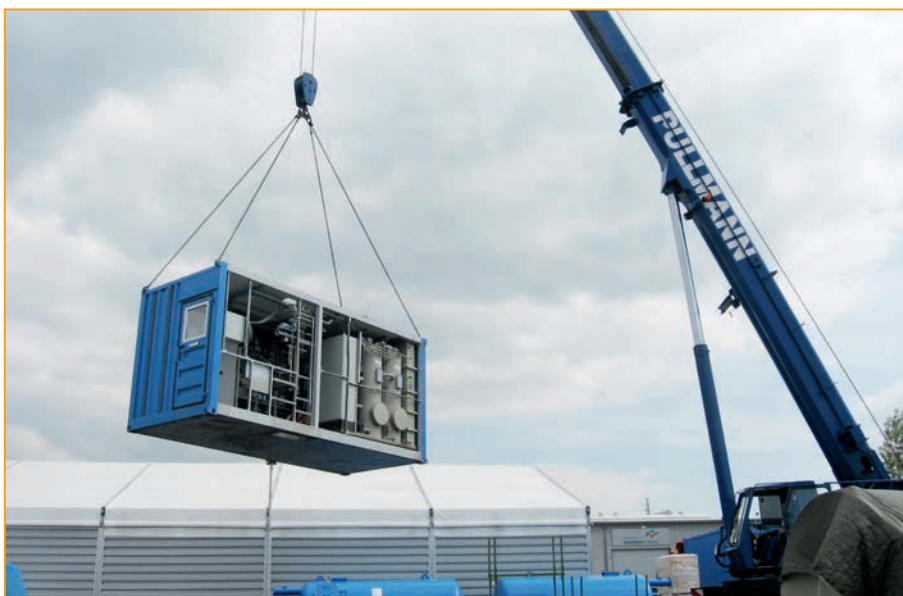
An EnviModul plant easily moved for wastewater treatment in the chemical industry.
