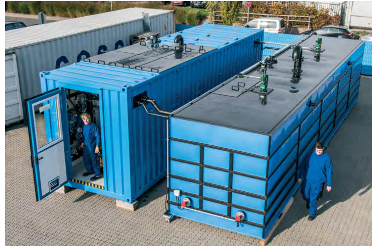
Pre-assembling of an EnviModul modular plant system with Biomar® OMB membrane biology
